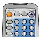
Distance: About 15ft from the front of the remote sensor. Angle: About 30 degrees in either direction relative to the remote sensor.
